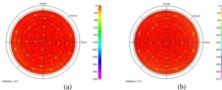
Figure 5. Experimental {200} pole figure ( $2\theta = 43.91^\circ$ ) of AlN\_C : (a) dcMS, (b) HiPIMS.
