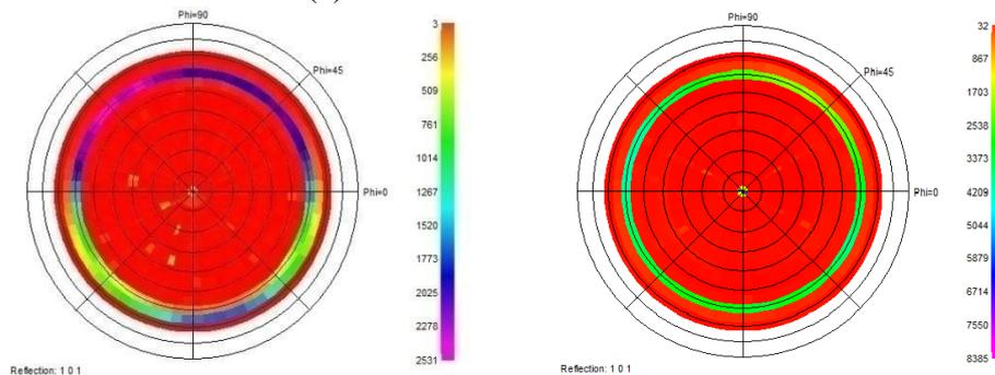
Figure 3. Experimental (10-11) ( $2\theta = 37.89^\circ$ ) pole figure of AlN\_H on: (a) AlN(2200nm)/Si(100), (b) AlN(1500nm)/Si(111)
