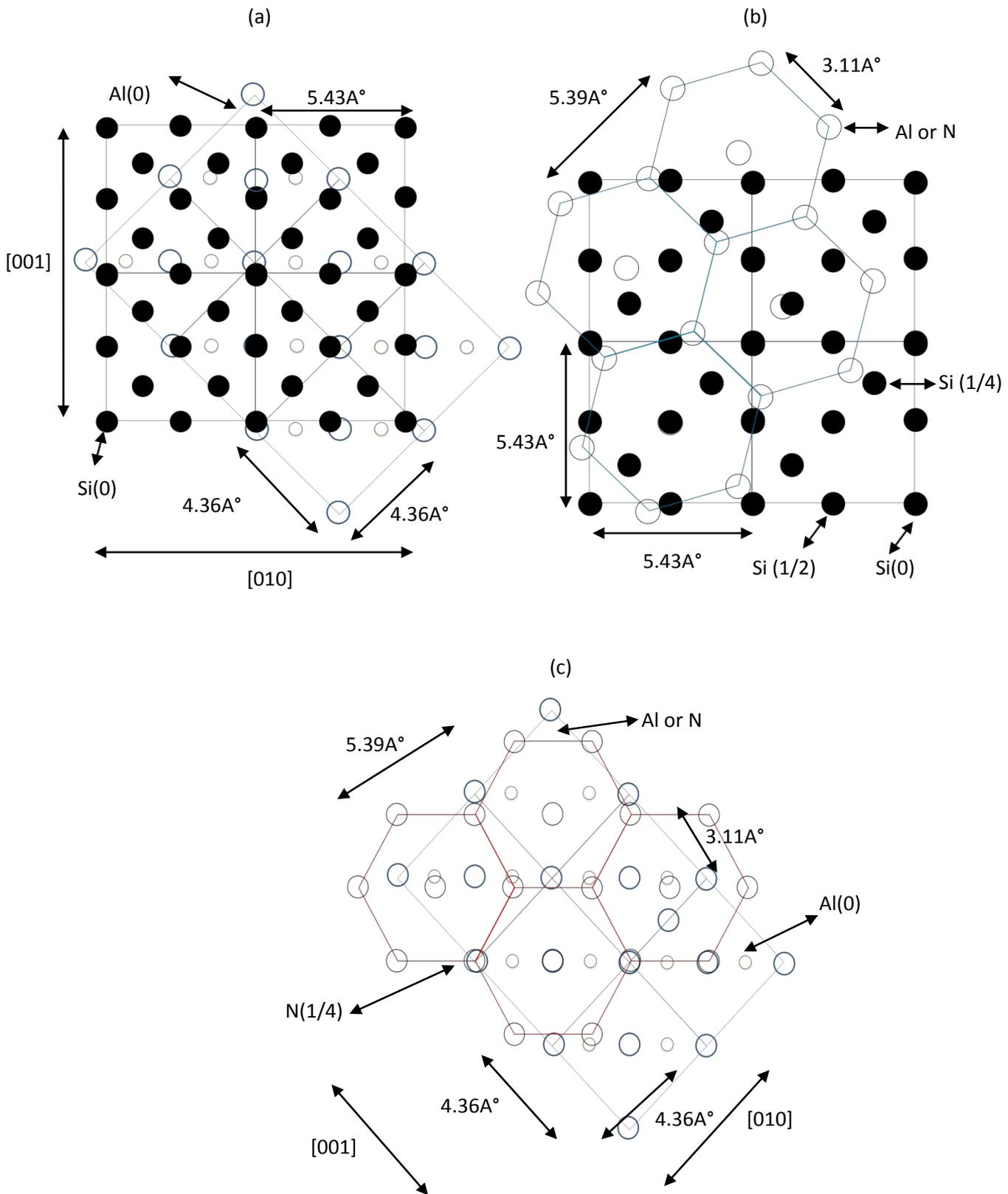
Figure.7. The atomic arrangements of (a) the epitaxial (100)AlN\_C/(100) Si interface, (b) the epitaxial (0001) AlN\_H/(100)Si interface and (c) AlN\_H(0001)/AlN\_C(100). ●Si, ○, N ○
