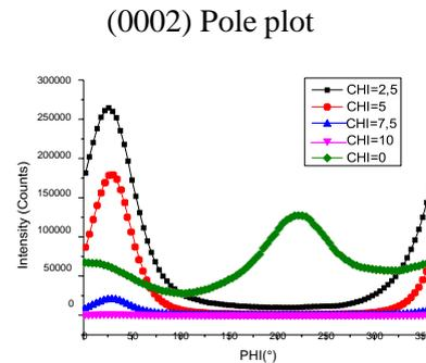
Figure 4. Intensity evolution report to azimuth angle PHI for CHI=0 to 10°
