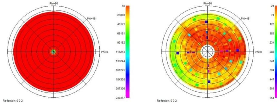
Figure 6. Experimental (0002) pole figure ( $2\theta=36.04^\circ$ ) of AlN\_H for HiPIMS method: (a) CHI=0 to  $75^\circ$  (b) CHI=15 to CHI= $70^\circ$ .
